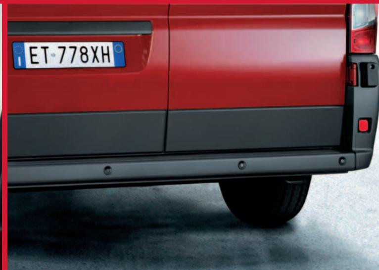
**Parking sensors.** The ultrasonic parking sensors are activated when reverse gear is engaged. An intermittent buzzer informs the driver of an approaching obstacle.
