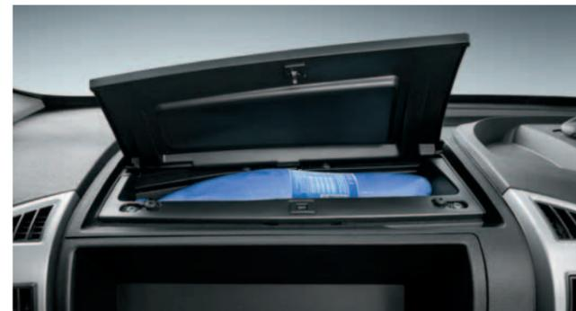
The refrigerated compartment keeps food and drinks cool when the air conditioning is in operation.
