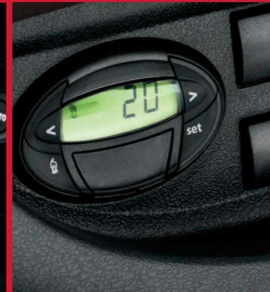
**Webasto.** Thanks to the programmable Thermo Top "C" Webasto heater, it is possible to heat the vehicle up to 24 hours before setting off. It can also operate instantaneously, heating the cab and engine and defrosting the windows. The system is also completely independent of the engine. The Webasto is also available in an automatic version without timer.
