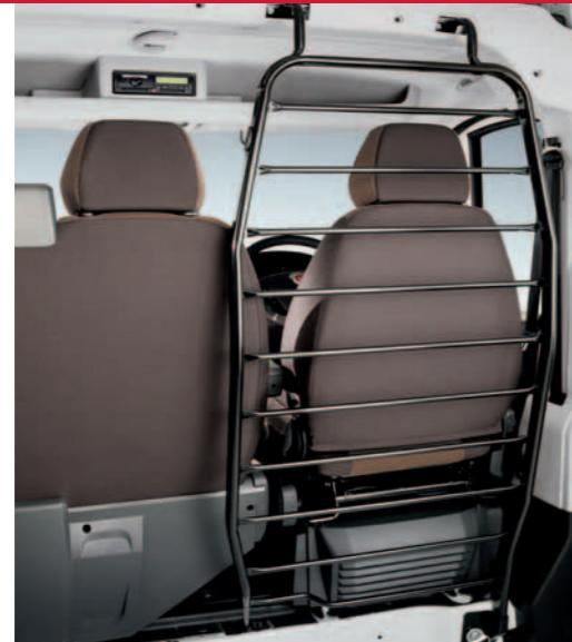
**Partitions.** The load compartment and cab are separated by a fully panelled metal partition. Available as an option, is a metal partition with window or a robust metal structure protecting the driver from the intrusion of transported material in the event of sharp braking.
