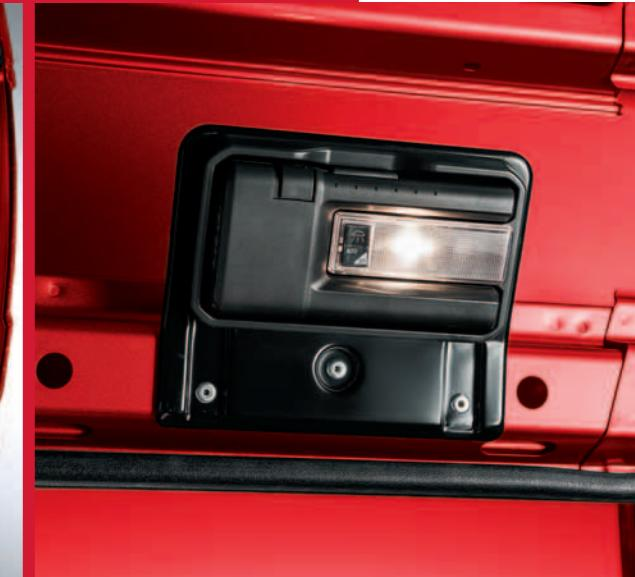
**Removable roof light.** The load compartment can be illuminated by a practical roof light which, when required, can be removed and act as a portable torch. Once returned to its housing, the torch will recharge automatically.
