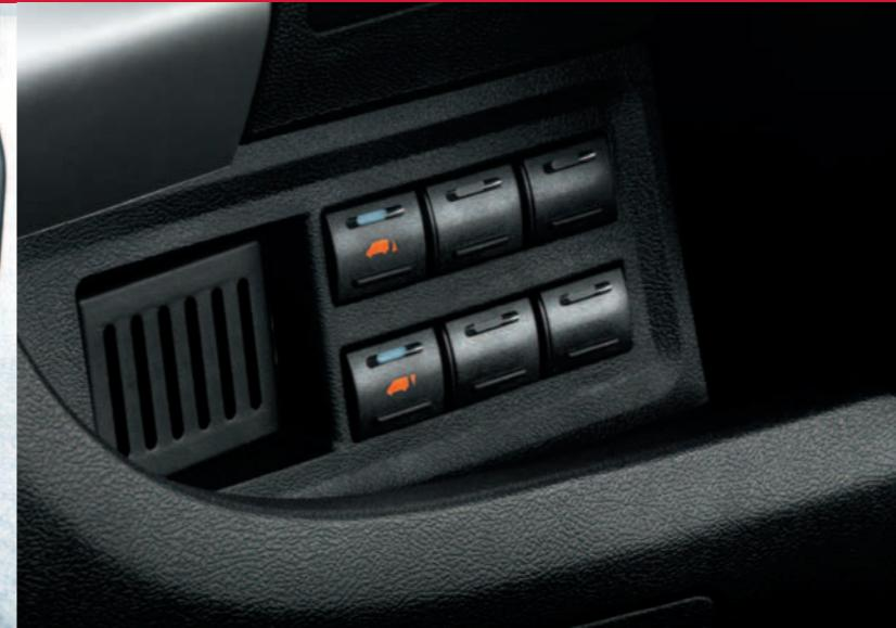
**Air suspension.** The air suspension enables the stability of the vehicle when driving to be maintained in all load conditions. With the vehicle stationary, the ground clearance can be increased or decreased to facilitate goods transport.
