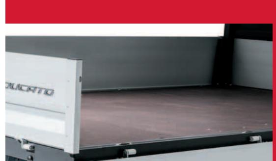
The load platform is lined with robust marine plywood.
