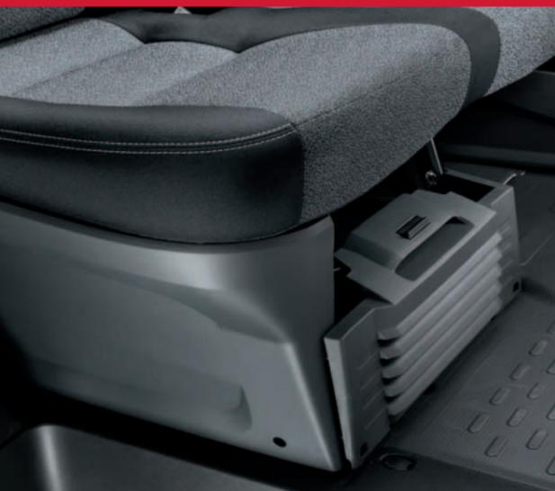
**Seat casing.** The casings conceal the seat supports and the storage compartments below the front seats.
