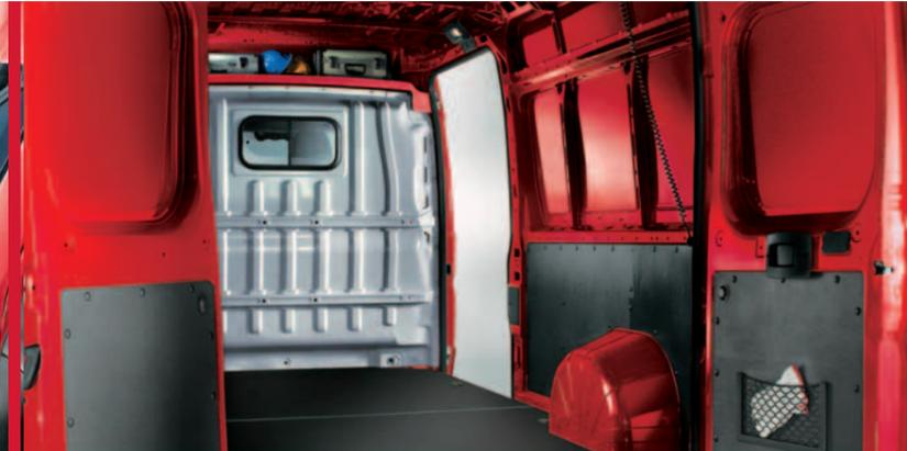
**Load compartment wall protections.** The walls of the compartment too can be lined with plastic protective panels. On request, panels are available up to mid-height or up to full roof height.
