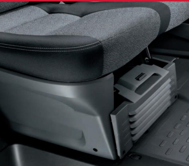
**Seat casing.** The casings conceal the seat supports and the storage compartments below the front seats.
